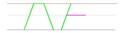
Mark out the tooth thickness again to locate a point on the other side of the gear tooth. Construct the side using the pressure angle.
