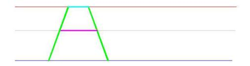
At this point construct a line using the *Pressure Angle*. From the starting point mark out the distance of the *tooth thickness:* Circular Pitch / 2 Circular Pitch =  $\pi$  (3.14) x m Using the same pressure angle contruct the remaining side of the gear tooth.
