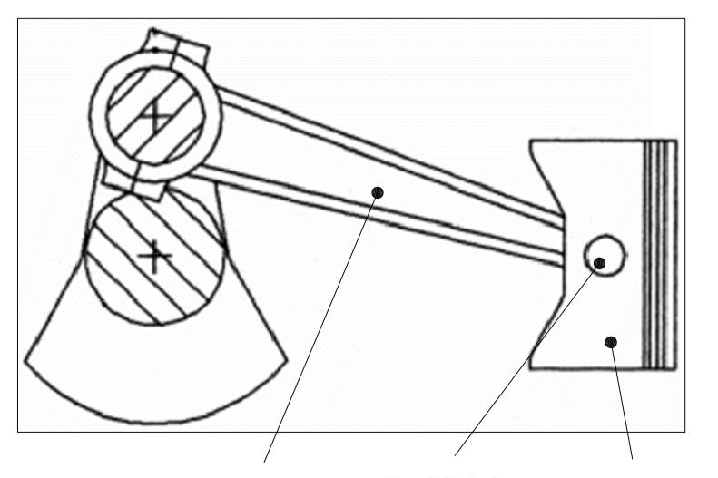
(i) A piston is a rigid, lubricated sliding shaft that fits tightly inside the opening of a cylinder. Its purpose is to change the volume enclosed by the cylinder.
