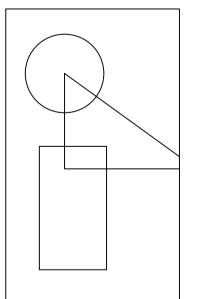
Zoom allows you to view a smaller area in more detail, or a larger area in less detail, without changing the drawings dimensions.
